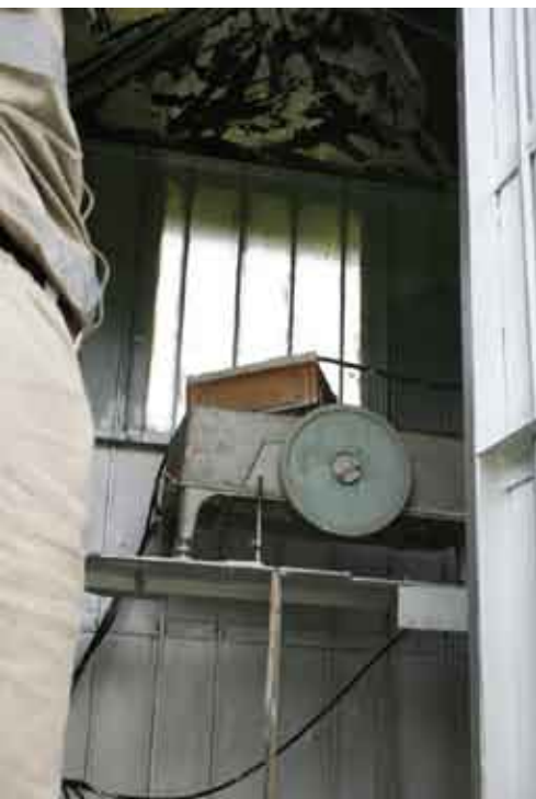
The old Stephens logger that has been in place for almost 50 years.
